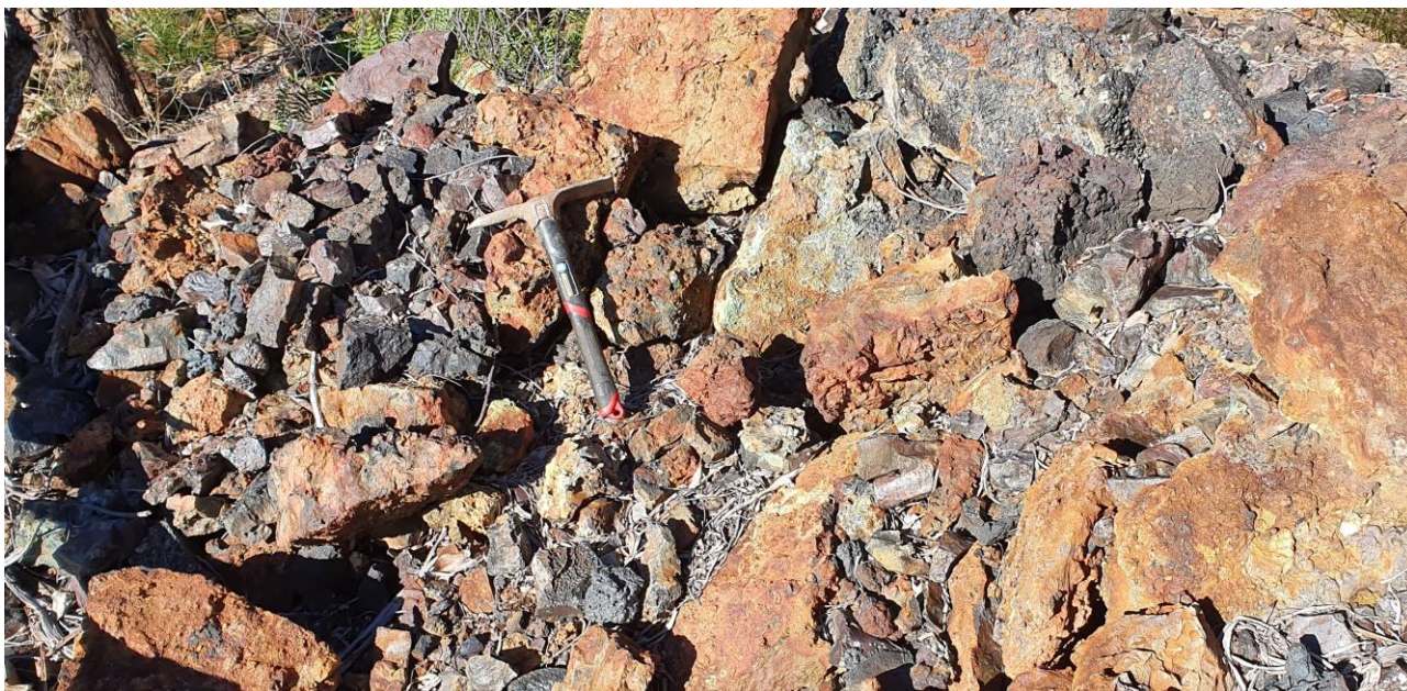
Figure 2: Slag close up. Light secondary copper (malachite) staining throughout
