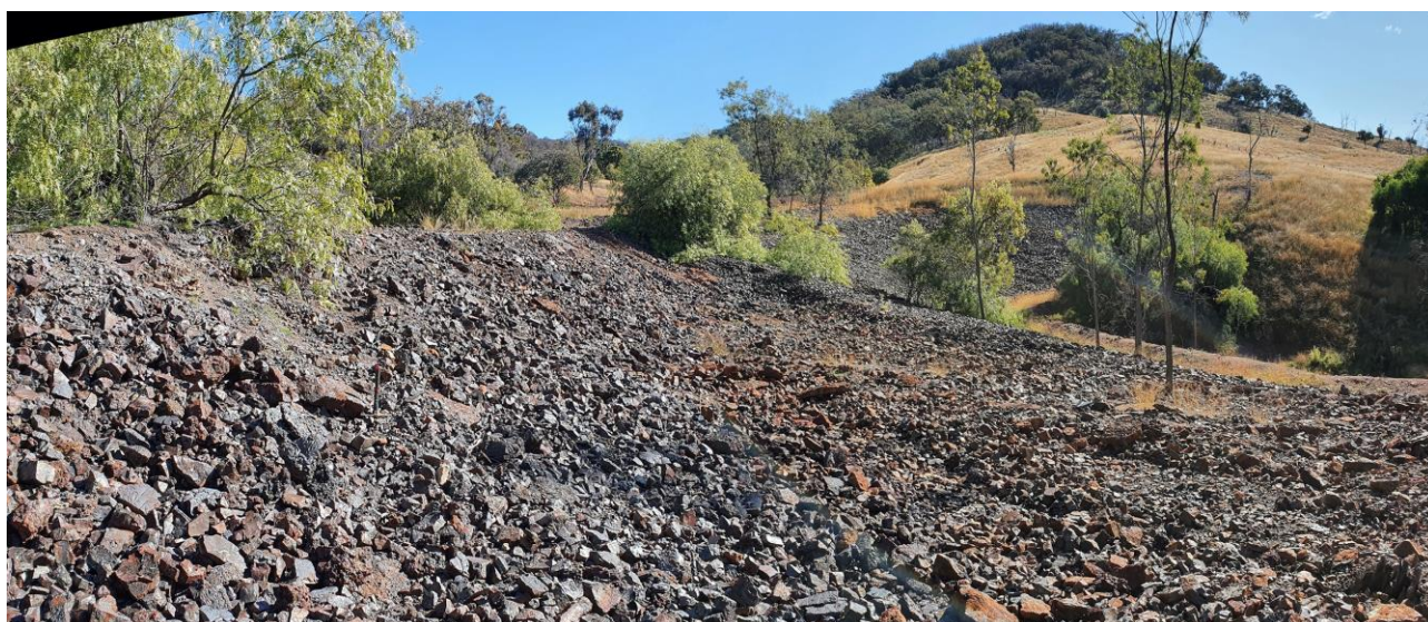
Figure 3: Looking westerly from the main smelting area located at the eastern end of the allotment. Slag has now been used as a “blanket” for sediment and erosion control purposes
